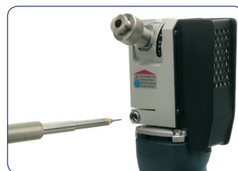
Precise adjustment of the stick-out
