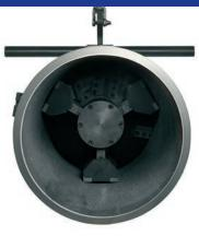
Innovative wide locking jaws offer 6 point locking from 3 jaws giving superior clamping force for chatter free end preps.
