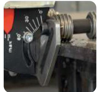
Continuous angle adjustment from 0 to 60 degrees.
