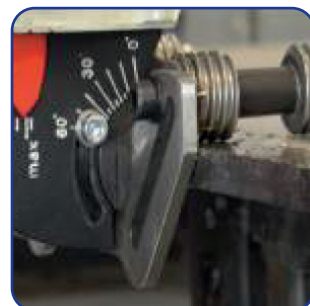
Continuous angle adjustment from 0 to 60 degrees.
