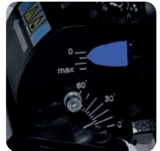
Continuous angle adjustment from 0 to 60 degrees.
