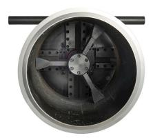
Innovative wide locking jaws offer 6 point locking from 3 jaws giving superior clamping force for chatter free end preps.
