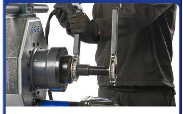
The PREP 24 has unrivalled power and stability, utilising a ratchet system for both jaw locking, and bevel feed.
